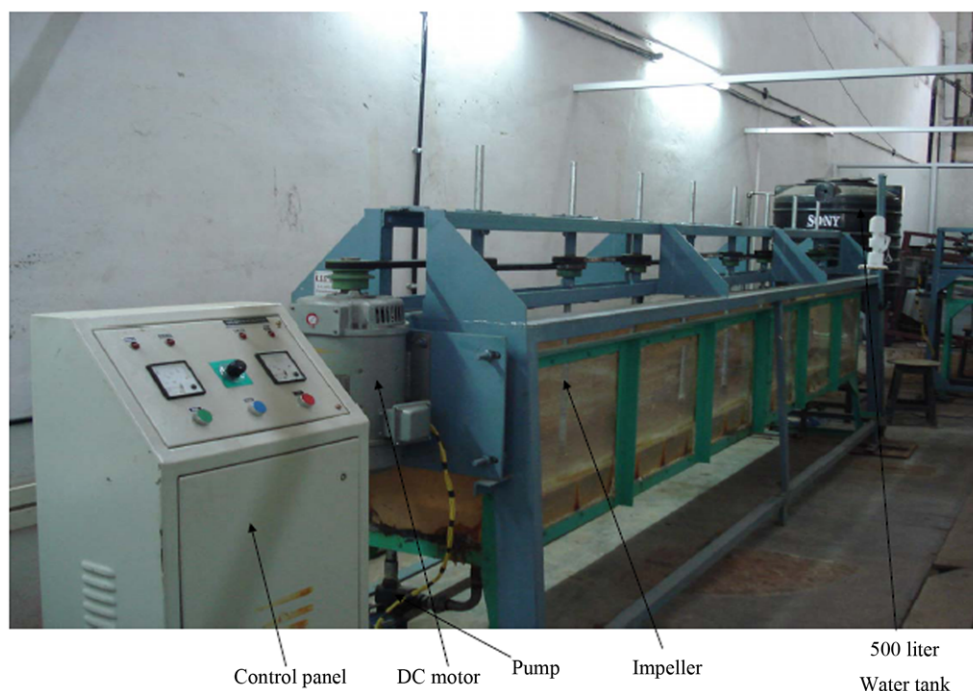
Fig. 2. Continuous flow surface aeration systems (40 cm×60×420 cm).
